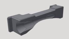
Component that guides the product and diverts it toward the hooking ring; once its wear threshold is exceeded it has to be replaced (1500-2000 ton.).
