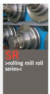
Various technical solutions are available for the multistrand straightening rolls located after cooling bed, in relation to product type and material quality.
